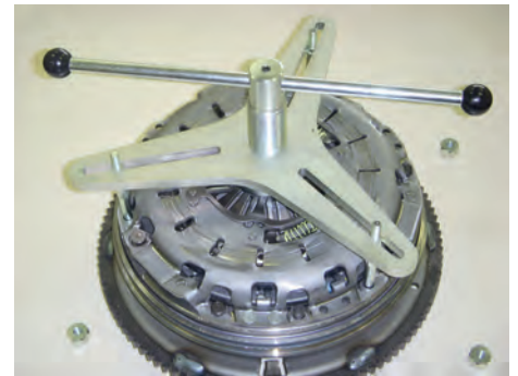
15. Loosen hexagonal nuts - remove clamping device.
