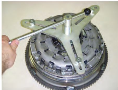
14. Completely turn back the pressure spindle - disc spring will release tension.
